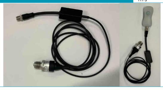
The pressure sensor measures line pressure in, for example, CO2, air or water lines. The pressure sensor is mounted with a straight male thread. The pressure sensor is connected to a FireFly.
