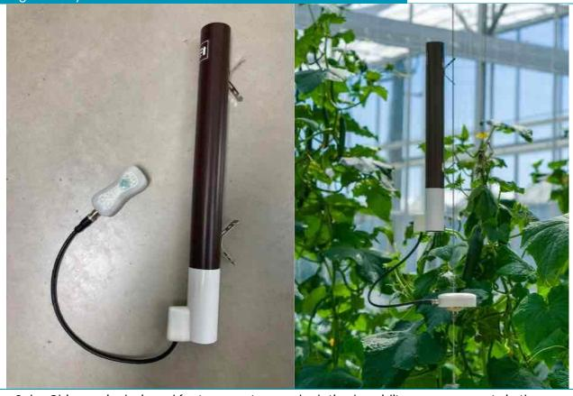
The Solar Chimney is designed for temperature and relative humidity measurements in the presence of high (solar) radiation. The radiation generates natural airflow through the chimney, allowing for ventilated air temperature and relative humidity. The FireFly platform sensor is connected via connector cable and provides data transmission. There are multiple mounting options to choose from. Use the Solar Chimney SubZero model for measurements below 0 °C (upon request).
