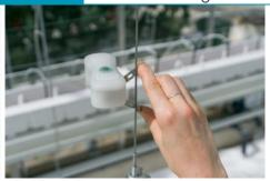
The clip can be used to mount the FireFly to a 2..3.5 mm diameter wire or a 6..7 mm diameter stick.
