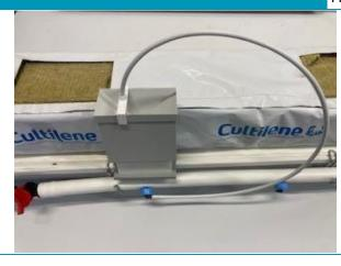
The sensor uses tipping-bucket (spoon) technology and measures: dripper or drain volume (flow rate), drain EC and drain temperature. The sensor connects to a FireFly.
