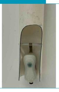
The clip allows the FireFly to be installed with a hook hanging vertically on a wire up to 6 mm in diameter. Among other things, this clip is used for mounting in the Macro Solar Chimney (L x D: 500 x 70 mm³, L x D: 19.7 x 2.75 inches³)
