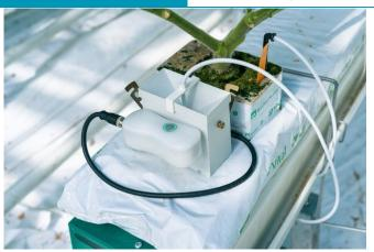
The sensor uses tipping-bucket (spoon) technology and measures dripper or drain volume (flow rate). The sensor connects to a FireFly.
