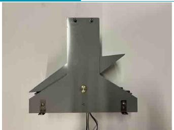
The drain/dripper sensor is a tipping-bucket sensor for measuring large drain volumes. The sensor connects to a FireFly.
