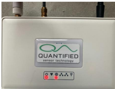
Figure 2: Correct lights for 4G-connection, wait +/- 5 minutes for lights to settle
