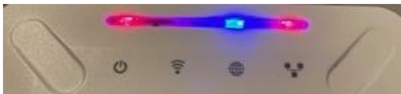
Figure 1: Correct lights (blue LED should not flash, wait +/- 5 minutes for lights to settle)
