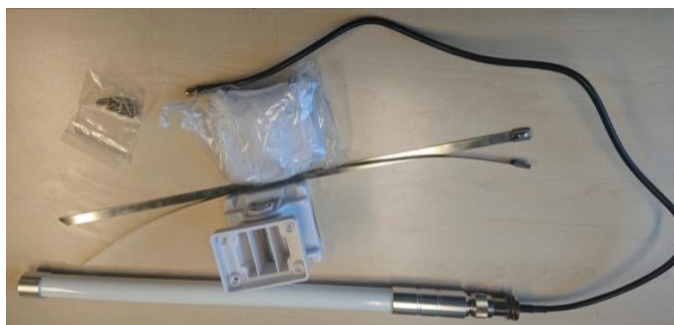
Figure 2: Mounting hardware and antenna
