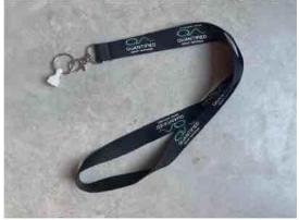
Magnet attached to a Quantified key cord for resetting the FireFly sensor.
