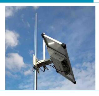
The solar outdoor 4G gateway receives LoRa messages from the FireFly sensors and sends the data over the Internet to the database. A single gateway is sufficient to process data coming from up to 100 FireFlies. Suitable for outdoor use, this GoutSolar gateway connects via a 4G connection and/or an Ethernet cable. The Gateway can be connected to the mains but also has a solar panel and battery to operate without a power connection.
