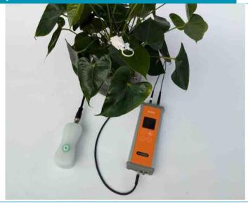
The Sendot Photo Efficiency sensor can be linked to the FireFly. This allows the sensor data to be read out digitally in the desired platform (including LetsGrow, Sendot and Ledgnd).
