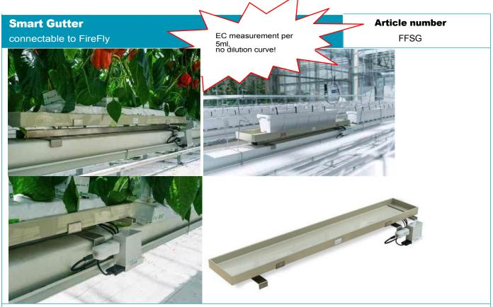
The Smart Gutter enables optimization of fertigation for cultivation in substrate slabs or multiple small pots (<20cm diameter). By measuring substrate weight, drain volume, drain EC (per 5ml!) and drain temperature every five minutes, the grower gains insight into plant evaporation and root climate. For high wire cultivation the Smart Gutter can be combined with hanging scales (see: crop weight monitor) for weighing the crop wires. With this
