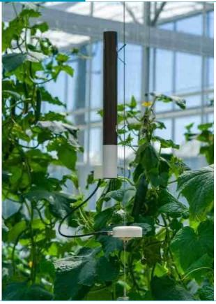
The Solar Chimney is designed for temperature and relative humidity measurements in the presence of high (solar) radiation. The radiation generates a natural airflow through the chimney allowing ventilated air temperature and relative humidity. The FireFly platform sensor is connected via connector cable and provides data transmission. There are several mounting options to choose from. Use the Solar Chimney SubZero model for measurements below
