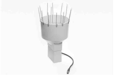
The pluviometer consists of a funnel with anti-bird prongs mounted on a "tipping bucket" sensor. The pluviometer measures precipitation in mm, and can be connected to a FireFly.
