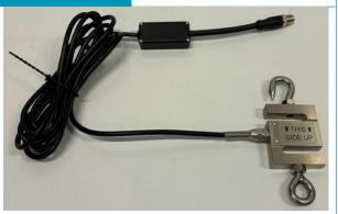
The hanging scale can be used for weighing hanging objects such as cultivation gutters or crop wires. The scale is available with various weight ranges. The scale connects to a FireFly and can be tared by wirelessly
