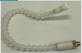
The Medusa T, rH is designed for targeted temperature and relative humidity measurements at limited space, for example between plants. The sensor head has a passively ventilated head that also provides protection against direct light irradiation.
