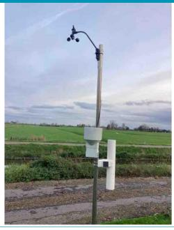
The weather station includes a wind gauge, pluviometer, air temperature and relative humidity. Optional features include a GPS module and a stainless steel pole.
