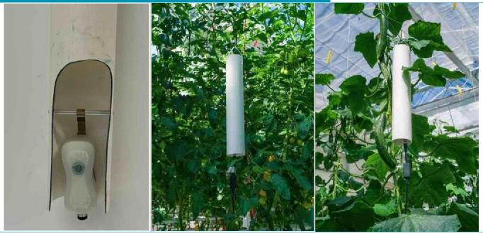
The Macro Solar Chimney is a passively ventilated housing for the FireFly. In environments with high irradiance (direct growth or sunlight), this housing provides more accurate measurement of temperature and relative air humidity. When using the Macro Solar Chimney, the PAR measurement is not usable because the light sensor is shielded.
