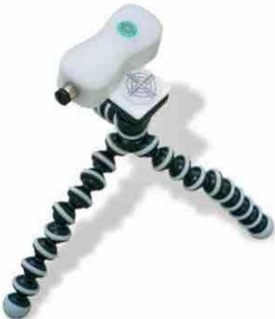
For level positioning of the FireFly for more accurate derived PAR light measurements.
