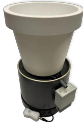
The Smart Gutter single pot makes it possible to optimize fertigation. By measuring substrate weight, drain volume, EC, and temperature every five minutes, the grower gains insight into plant evaporation and root climate. The EC is measured per 5 ml of drain, which means there is no delaying dilution curve and the EC response is very fast.
