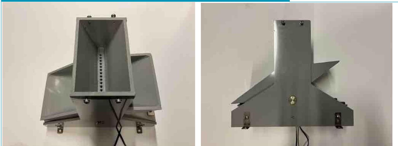
The XXL drain/dripper sensor is a tipping bucket for measuring discharge volumes between 0.5 and 25 liters/min. The sensor is connected to a FireFly.
