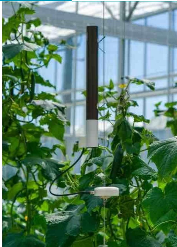
The Solar Chimney is designed for temperature and relative humidity measurements in the presence of high (solar) radiation. The radiation generates a natural air flow through the chimney, enabling ventilated air temperature and relative humidity measurements. The FireFly platform sensor is connected via the connector cable and provides data transfer. There are several mounting options to choose from. Use the Solar Chimney SubZero model for measurements below 0 °C (on request).
