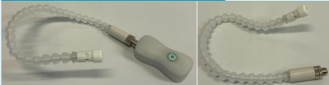
The Medusa T, rH is designed for microclimate temperature and relative humidity measurements between plants. The sensor head has a passively ventilated head that provides protection against direct light exposure.
