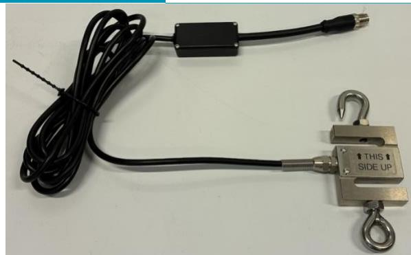
The hanging scale can be used to weigh hanging objects such as growing gutters or crop wires. The scale is available for various measuring ranges. The scale is connected to a FireFly and can be tared by resetting the FireFly wirelessly
