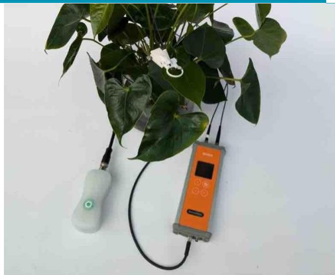
The Sendot Photosynthesis Efficiency sensor can be connected to FireFly. This allows the sensor data to be read digitally in the desired platform (including LetsGrow, Sendot, and Ledgnd).
